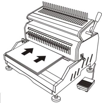
1. Align **Side Margin Control** to proper sheet & cover size.
