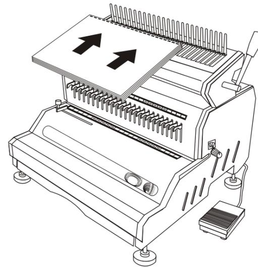
1. Place pre-selected comb behind Comb Binding Fingers. The comb opening side should be upward.
